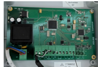
Terminals connecting input signals
